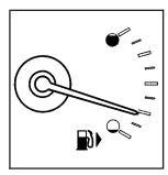
The fuel gage shows approximately how much fuel is in the fuel tank. It works only when the engine is on. All of the following situations are normal and do not indicate that anything is wrong with the fuel gage:
